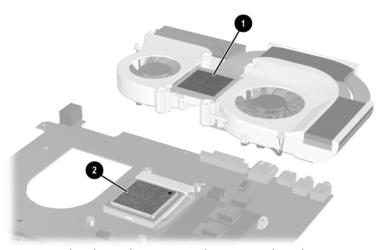
Removing the Thermal Paste From the Heat Sink and Processor Reverse the above procedure to install the heat sink.
